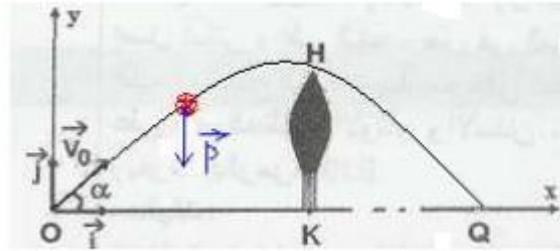
$$\vec{V}_0 \begin{cases} V_{0x} = V_0 \cdot \cos \alpha \\ V_{0y} = V_0 \cdot \sin \alpha \end{cases}$$
