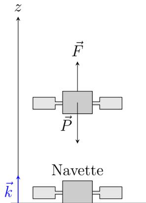
$$\begin{aligned} \sum \vec{F} &= m\vec{a} \iff \vec{F} + \vec{P} = m\vec{a} \\ &\iff F - P = ma \\ &\iff a = \frac{F - mg}{m} \\ &\iff a = \frac{F}{m} - g = C^{\text{te}} \end{aligned}$$
